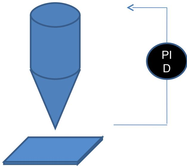
Measures a quantity  $F$  that is fed into a PID. This determines the difference to a desired value and changes the position of the tip accordingly, using an actuator.
