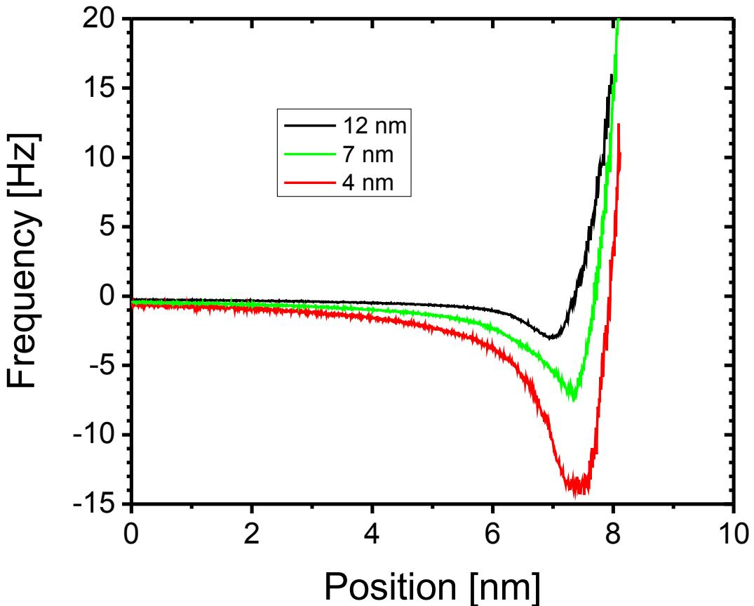
The observed change in resonance frequency with distance can be of the order of 10 Hz. Our resonance had a width of 0.2 Hz, making constant frequency excitation impossible.
