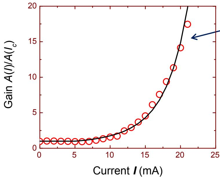
Theory  $G(I/I_c) = \exp\left[a\left(\frac{b_1 I + b_2 I^2}{b_1 I_c + b_2 I_c^2} - 1\right)\right]$
