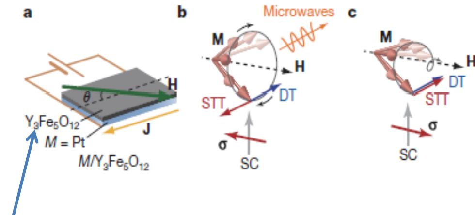
**YIG-Yttrium Iron Garnet** is a ferrimagnetic insulator with very small magnetic losses
