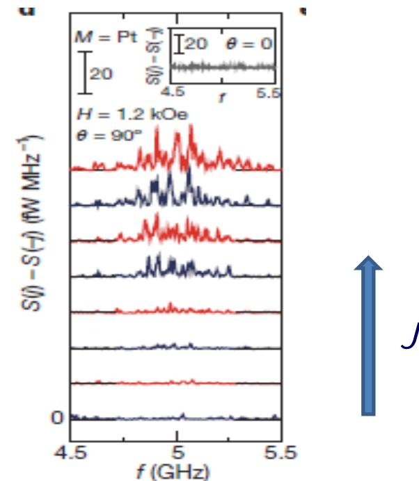
Excitation of spin waves by the spin-torque due to spin current created through the spin Hall effect
