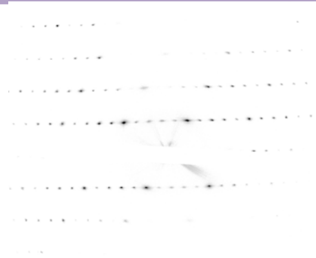
diffraction pattern of single nanowire
