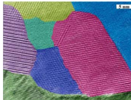
ZT~1.4 @ 373 K bulk – fine grain p-type, (Bi,Sb) 2 Te 3 [15 authors, BC/MIT/GMZ Energy/Nanjing University, 2008]
