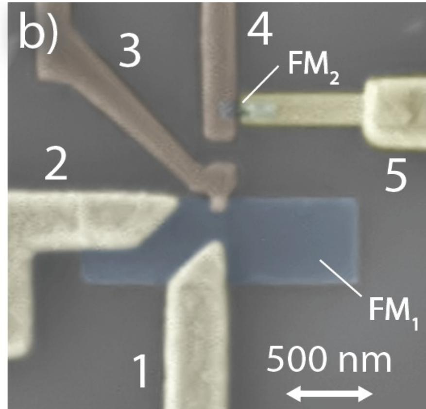
Current from 1 to 3, voltage measured between 4 and 5
