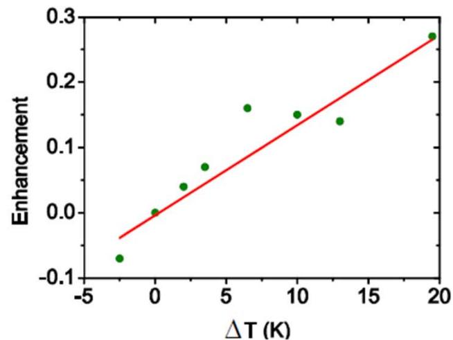
**Enhanced FMR peak amplitude upon the application of a temperature gradient**
