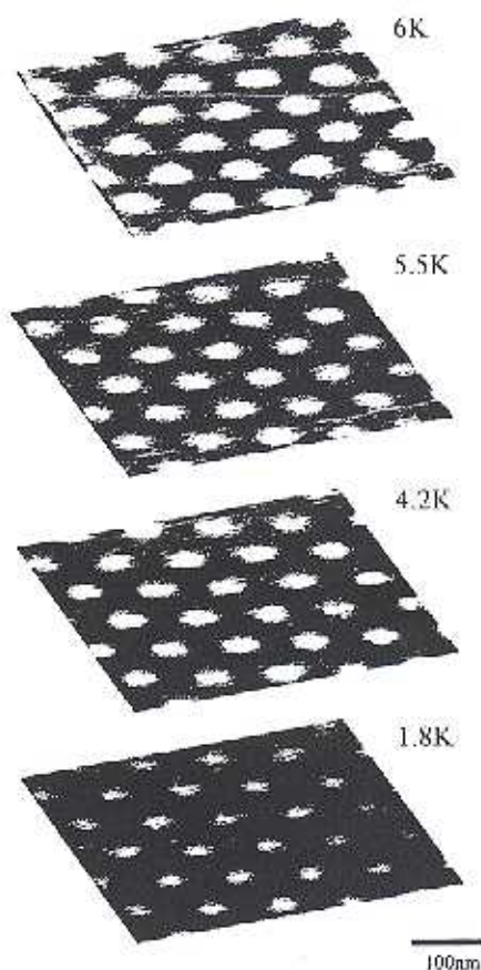
Fig. 2. Vortex lattice images measured at V_b = 0.5 mV, at different temperatures as indicated.
