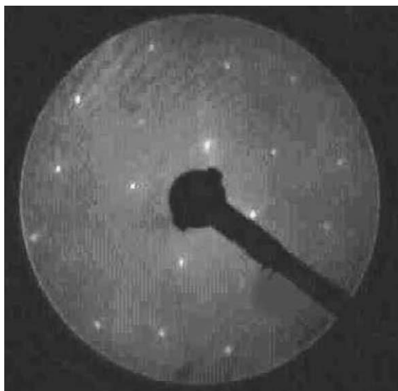
Fig. 1. The LEED pattern measured at room temperature with an electron energy of 193 eV for a \text{Sr}_2\text{RuO}_4 sample cleaved at T = 8 K.
