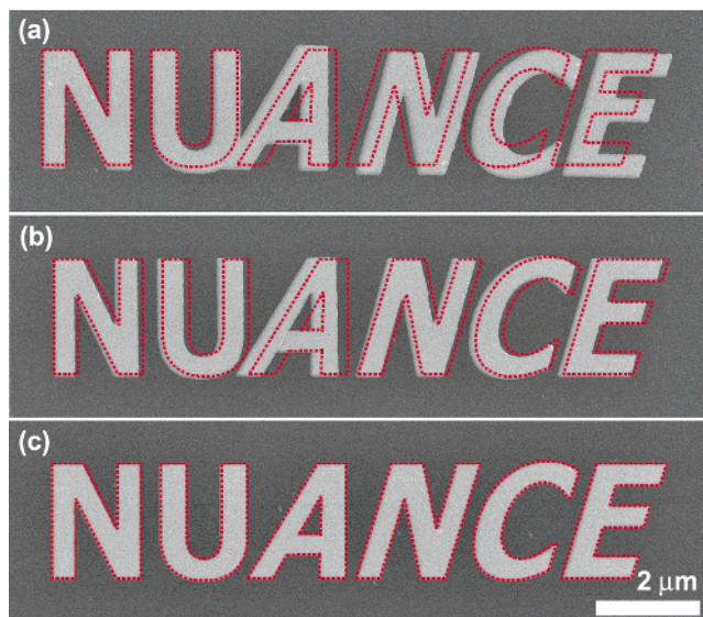
Figure 1. VPSEM images of 15 nm Au/Pd film patterned on a glass substrate with a 30 keV primary beam energy under (a) high vacuum, (b) 0.4 Torr, and (c) 1 Torr. The dashed red line indicates the pattern dimensions as written. The letters N, U, N, C, and E were patterned in order, followed by A in order to highlight the charging-induced pattern displacement. The pattern exposed using the VP- e BL process with 1 Torr chamber pressure shows no significant distortion or displacement.
