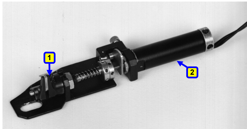
Figure 15-16: Clamp Assembly for 90° Wire Feed
