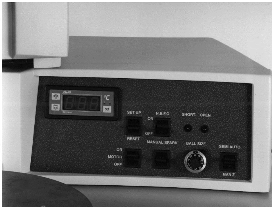
Figure 4-3: Right Control Panel - 4522, 4524
