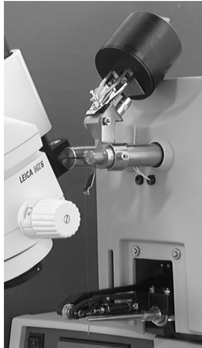
Figure 3-2: The Main Head Assembly – 4523, 4526
