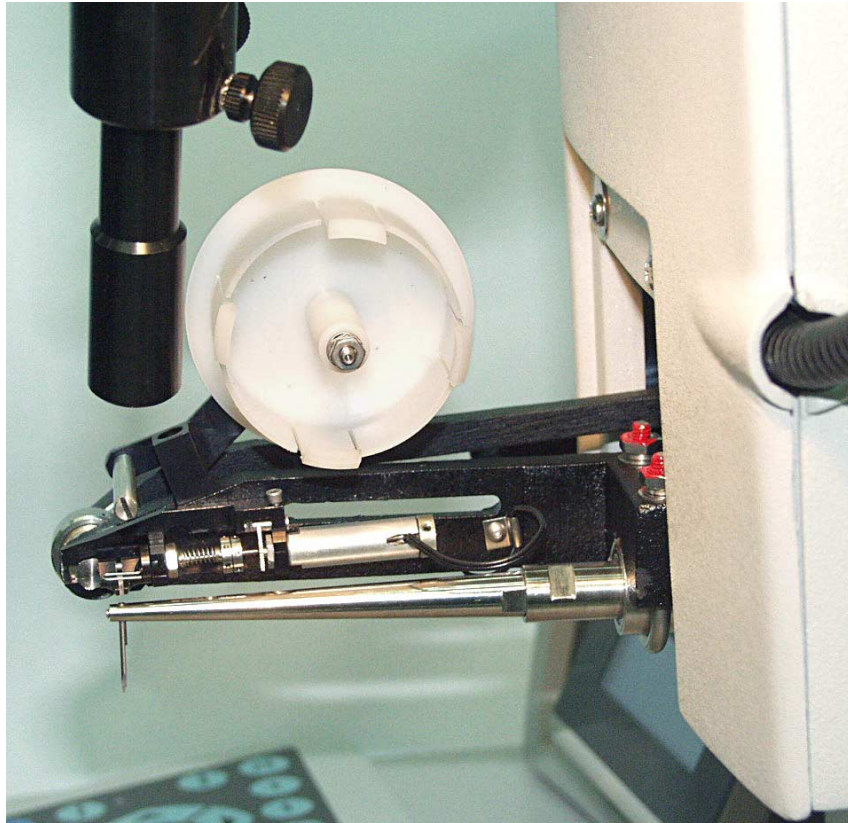
Figure 5-12: Close-up of 2" Spool for Ribbon Wire Vertical Feed
