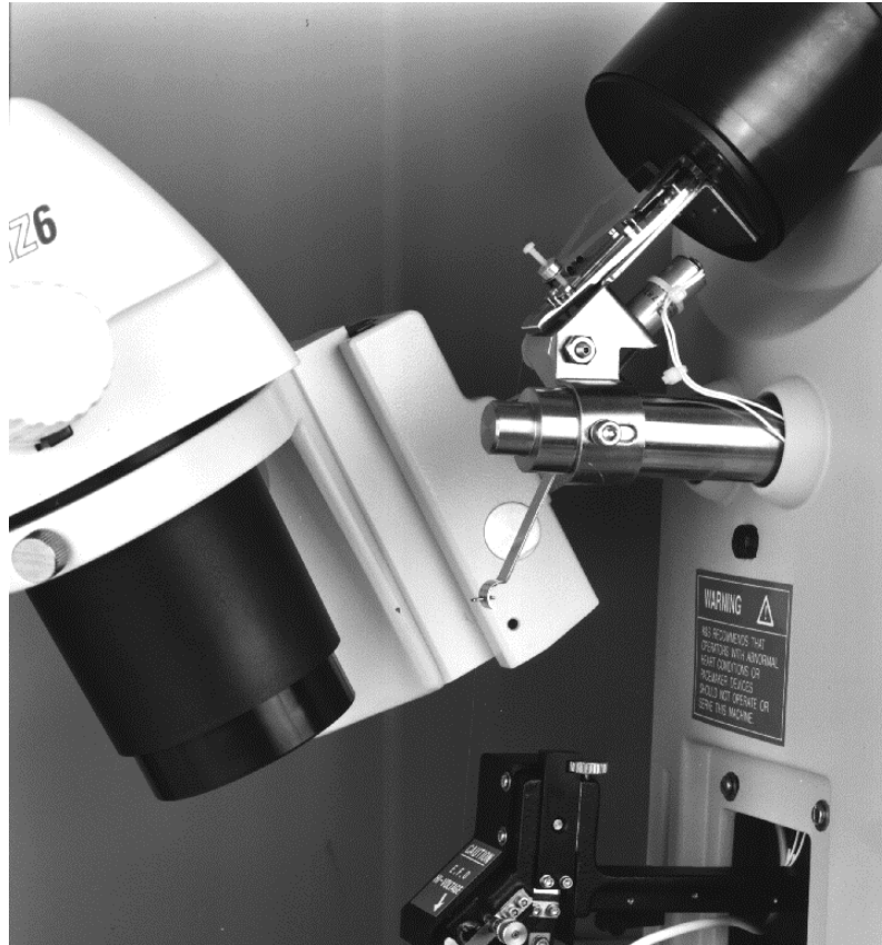
Figure 5-5: Wire Loading of 2" Spool - Vertical Wire Feed
