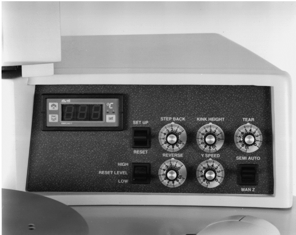
Figure 4-5: Right Control Panel - 4526
