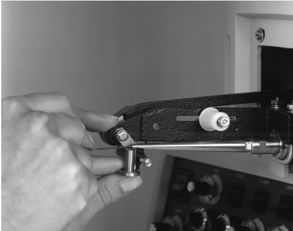
Figure 5-1: Wedge Installation Using the Setup Gauge - 4523, 4526 with 30°/45° Wire Feed, 0.75" Drop
