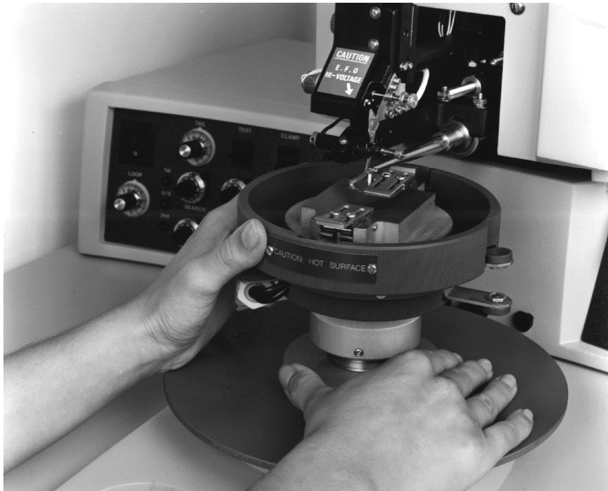
Figure 5-4: Adjusting Workholder Height
