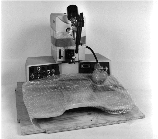
Figure 2-6: K&S 4500 Wire Bonder on Shipping Board
