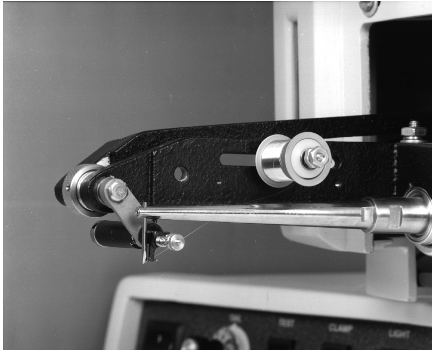
Figure 5-6: Wire Loading of 0.5" Spool - 30°/45° Wire Feed
