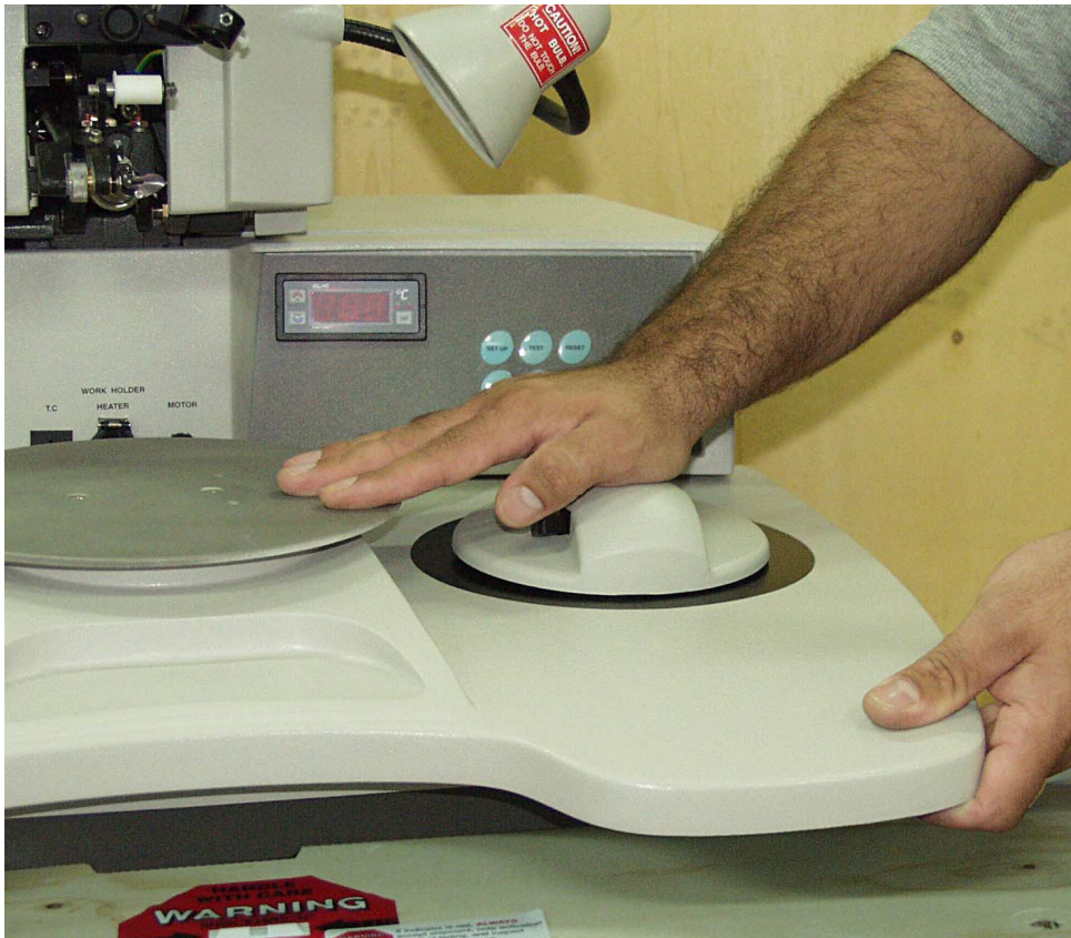
Figure 2-10: Support the chessman and manipulator and lift
