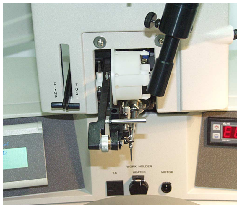
Figure 5-11: 2" Spool for Ribbon Wire Feed
