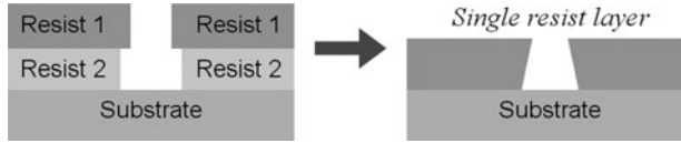
Fig. 2.18 Undercuts created in PMMA by using low-kV EBL enables replacement of bi-layer resist schemes ( left ) with a simpler single-resist layout ( right )
