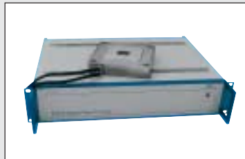
E-710.6CD 6-axis digital piezo controller shown with custom Super Invar 6-DOF piezo flexure NanoPositioning stage (110 V, 25 W, 3 to 6 Channels). See PI Catalog
