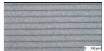
Layers in cofired monolithic piezoelectric actuator
