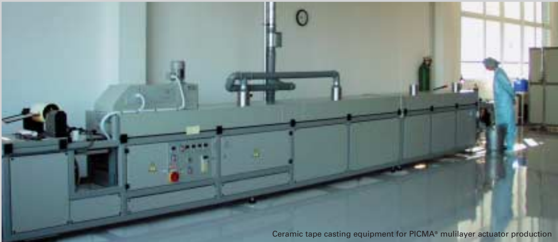
Ceramic tape casting equipment for PICMA® multilayer actuator production
