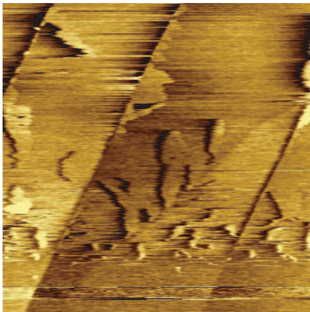
Figure 3.6: TM height image: 5.2 \times 5.2 \mu\text{m}^2 . As the RH is raised to 80% the surface appears to be 'flooded'.
