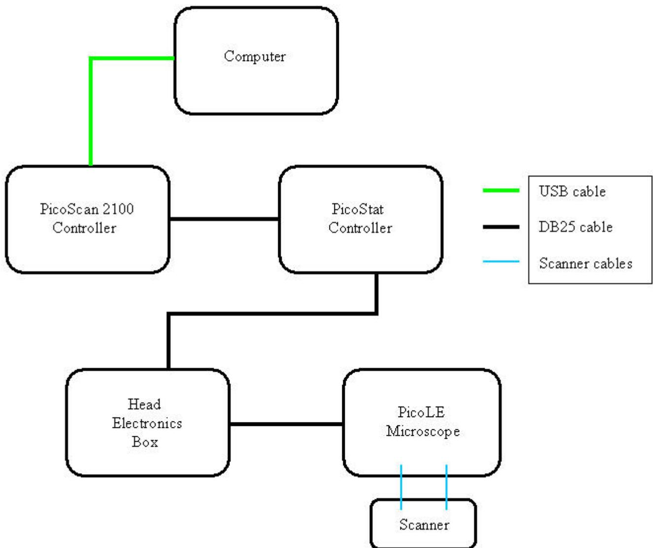
**Connection Diagram for a PicoLE System with PicoStat and AC Mode Controller**
