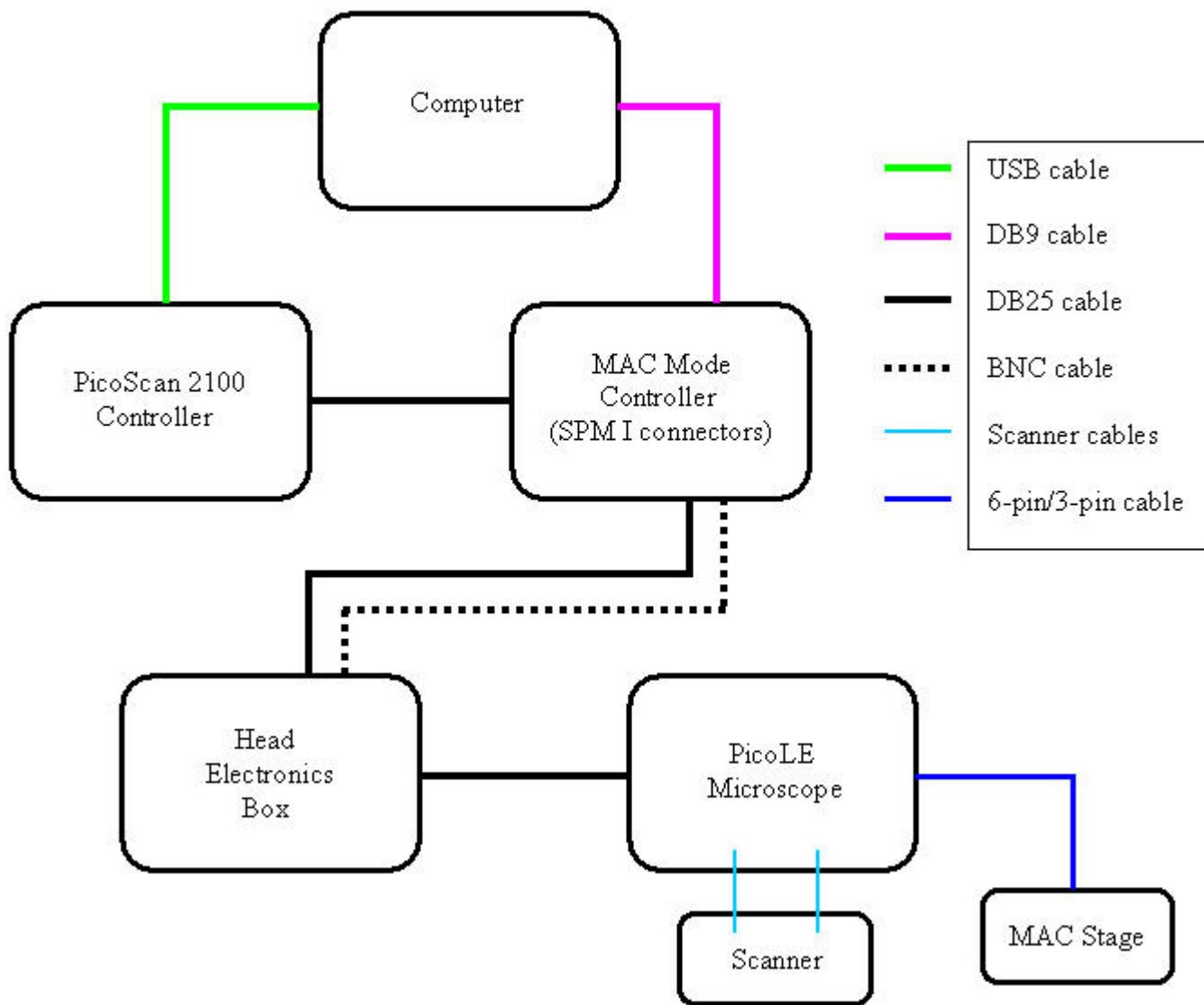
**Connection Diagram for a PicoLE System with PicoStat**
