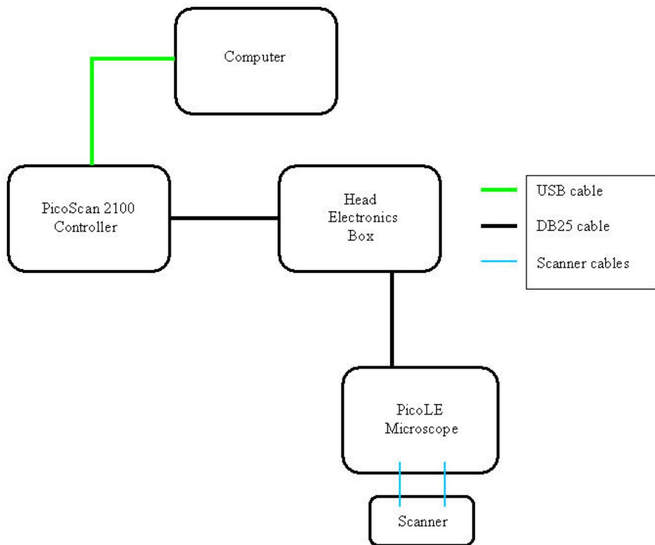
**Connection Diagram for a PicoLE System with an AC Mode Controller**
