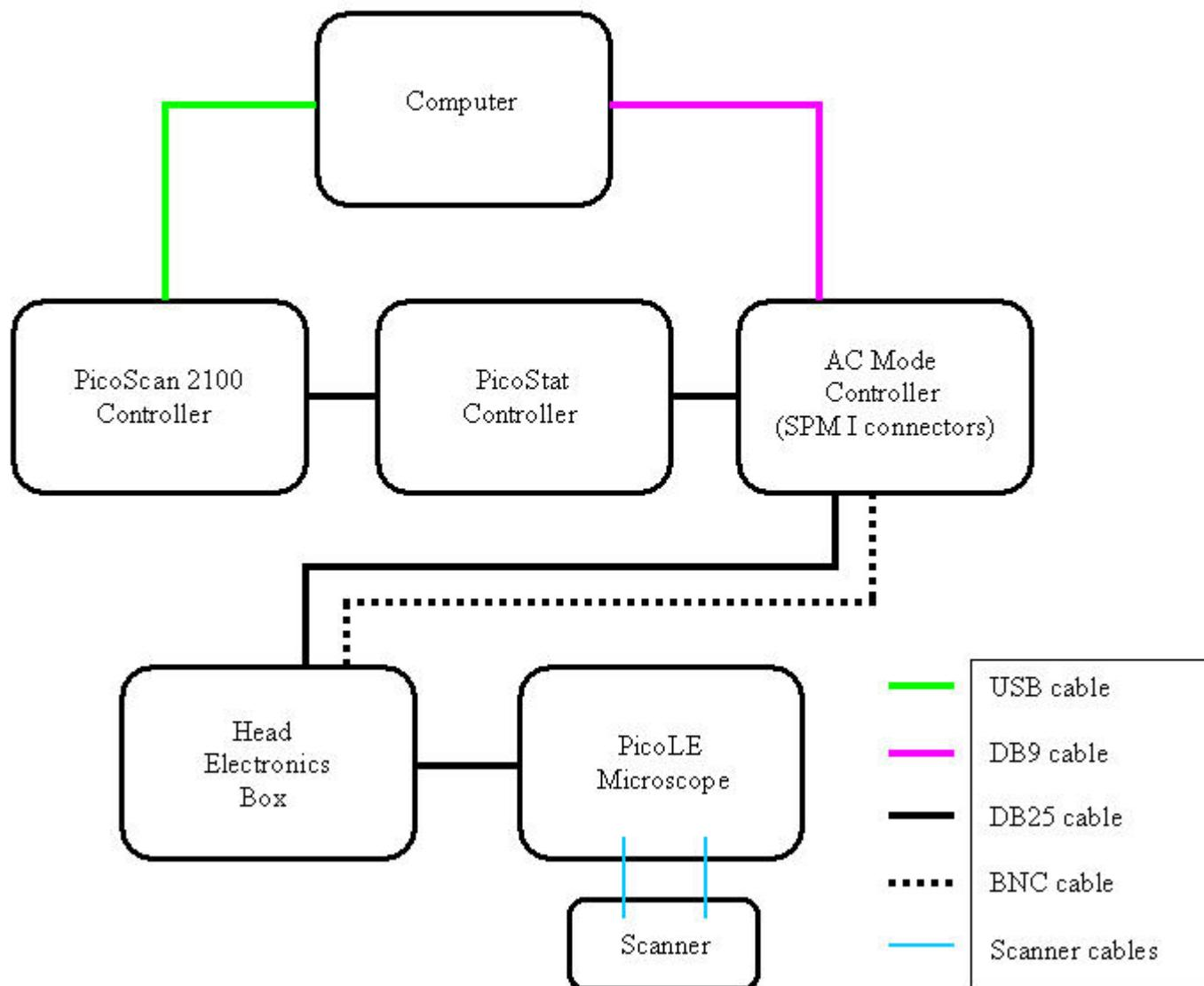
**Connection Diagram for a PicoLE System with PicoStat and MAC Mode Controller**
