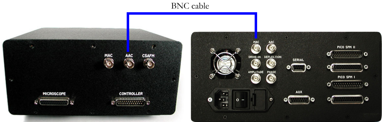
Figure 5 (left: PicoLE Head Elec. Box, right: MAC Mode Controller)
