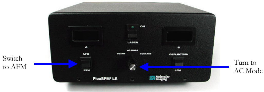
Figure 4 (Front of the PicoLE Head Electronics Box)
