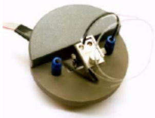
Shear Force head for SNOM
