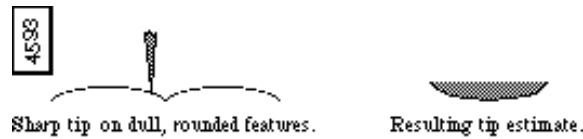
Figure 14.9e A sample with no sharp features yields a dull tip estimate.
