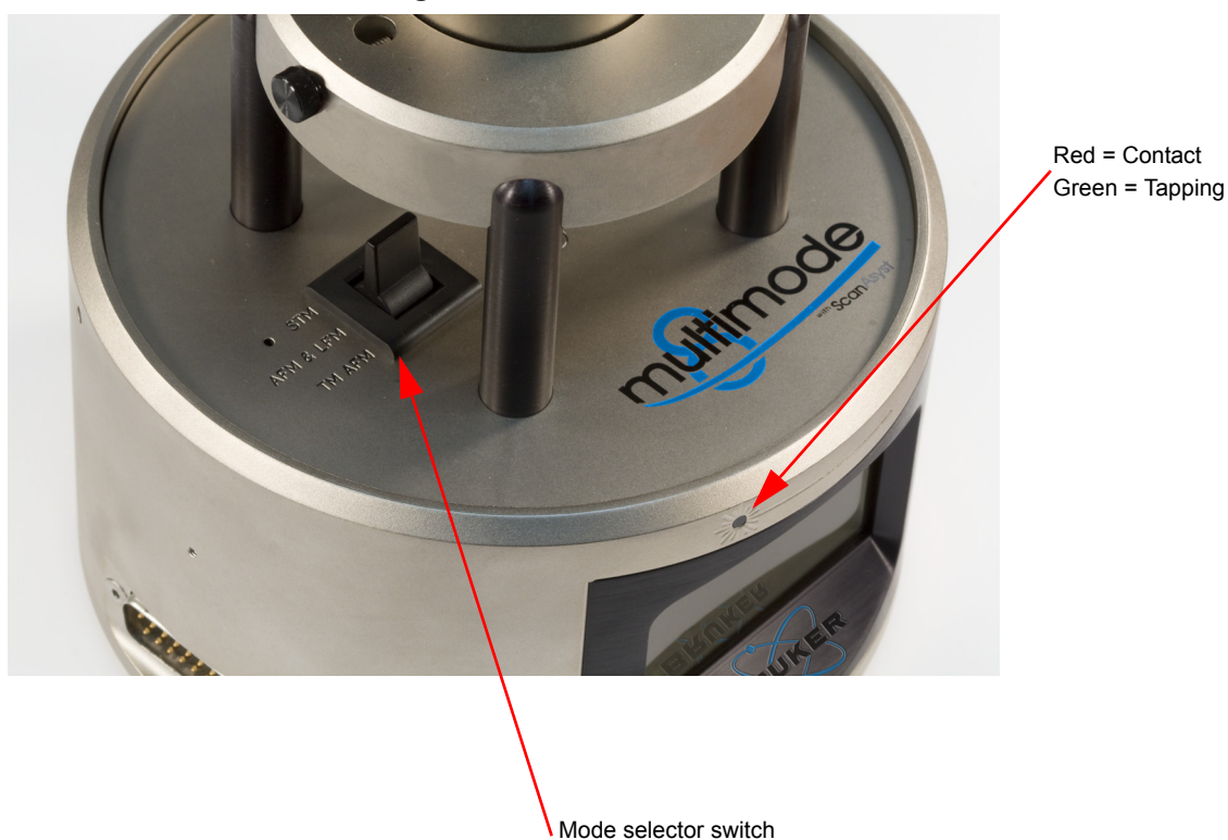
Figure 8.4a Mode selector switch
