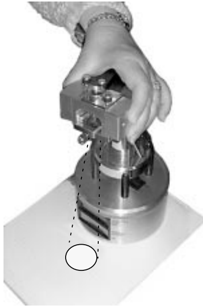
Figure 5.17. Projecting diffraction patterns downward with head removed. NOTE: Microscope shown is a MultiMode™ AFM, however, procedure applies to all current models of small sample microscopes.
