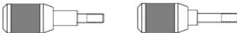
Figure 15.8. Stabilizing screw for securing the vertical scanner to the support ring. MultiMode AFM screw (left), and screw for other SPMs (right).
