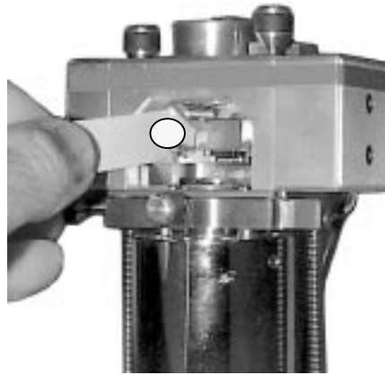
Figure 5.10. Paper method of laser alignment using a slip of paper inside SPM head.
