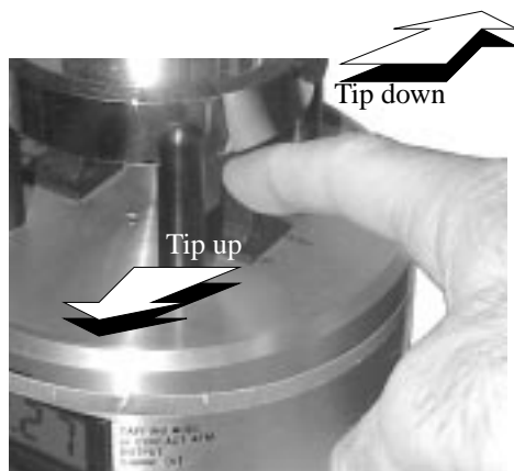
Figure 5.4. The tip is quickly raised and lowered using the Up / Down toggle switch on the MultiMode SPM's base.
