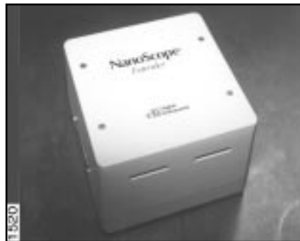
Figure 14.2. Extender™ Electronics Module—required for frequency phase detection MFM and EFM.
