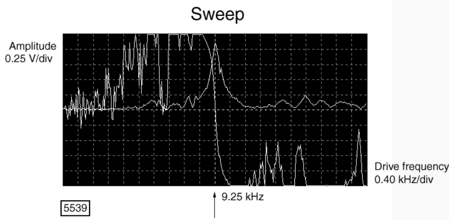
Figure 8.3a A 100 \mu\text{m} , Narrow-legged, Si 3 N 4 Cantilever Fluid Tune Curve
