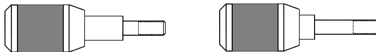
Figure 15.16b Stabilizing screw for securing the vertical scanner to the support ring. MultiMode AFM screw (left), and screw for other SPMs (right).
