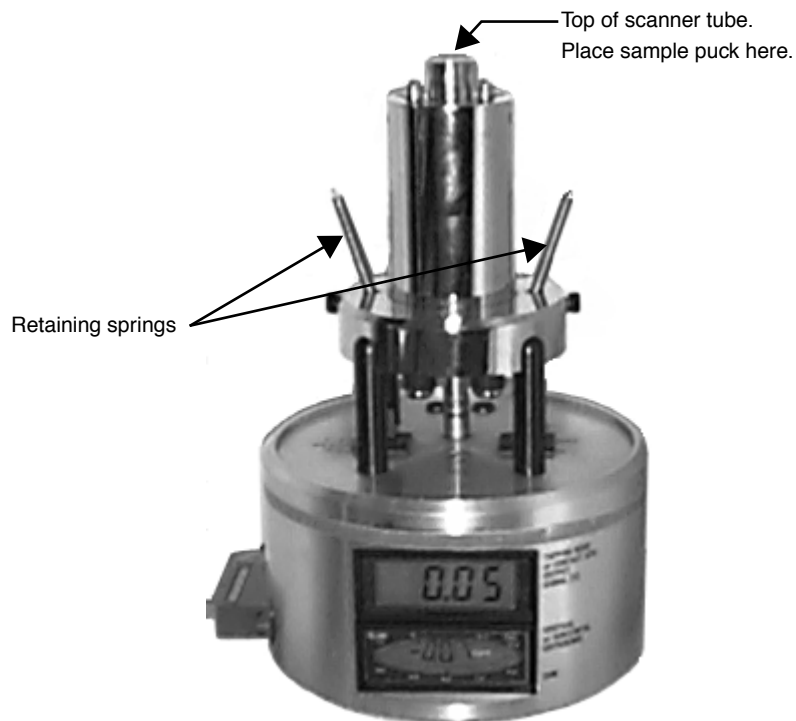
Figure 5.1b MultiMode Base with Scanner Mounted on Support Ring
