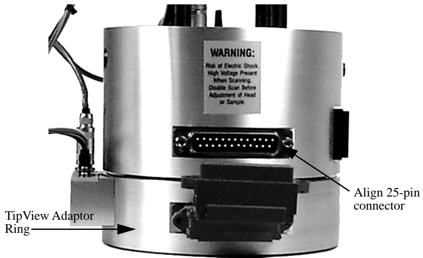
Figure 232-4 Place AFM base on the TipView adapter ring.
